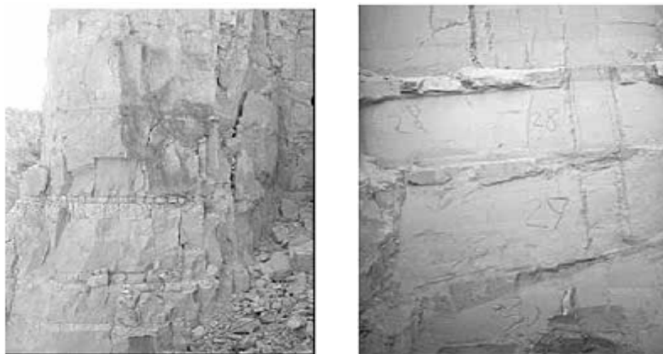
Fig. 2 Distinct layers in the vertical sediment profile upstream of the warping dam caused by rainstorm events.
