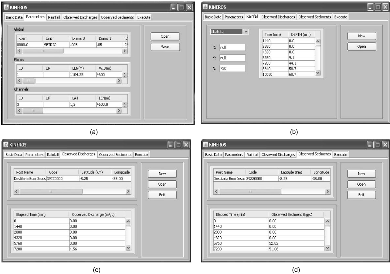
Fig. 3 Graphical user interfaces of the model input data: (a) input parameter data (step 2), (b) rainfall data (step 3), (c) observed runoff (step 4), and (d) observed sediment yield (step 5).
