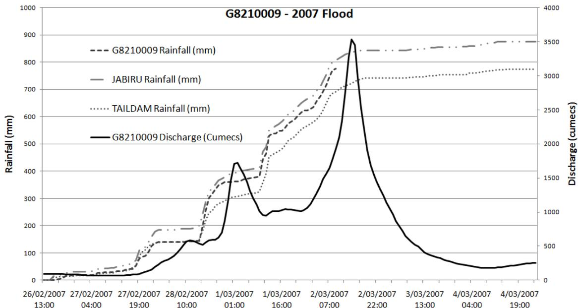
**Fig. 2** Mass curves of rainfall at gauge G8210009, Jabiru Airport and Ranger Tailings Dam, and flood hydrograph at Magela Creek at G8210009.
