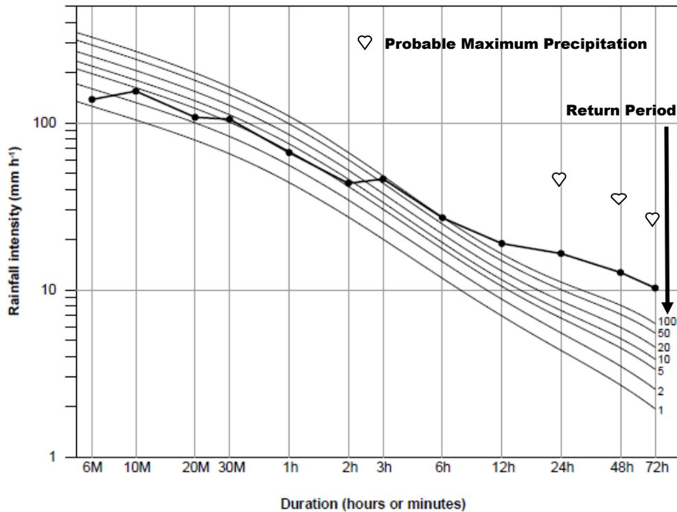
**Fig. 3** Rainfall intensity-frequency-duration curves for G8210012 derived by the Bureau of Meteorology with the recorded rainfall for G8210012 shown in bold and PMP shown by hearts.
