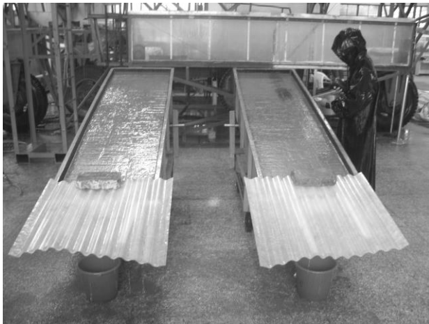
Fig. 1 The artificial unmetalled loess road sections, showing flow velocity measurement using a dye tracing technique.
