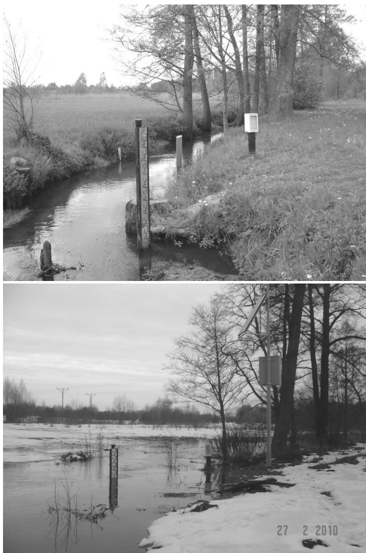
Fig. 2 Views of the gauging station at Plachty Stare (photos are looking downstream: top photograph – during a low flow period in May 2006; bottom – during a snowmelt period in 2010, when the discharge was close to the 2-year flood).
