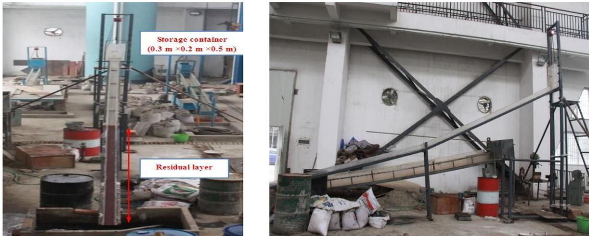
Fig. 4 Frontal and side views of the flume.
