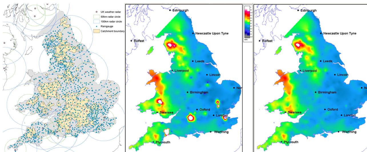
**Fig. 2** Distribution across England and Wales of raingauges, weather radar and catchments used in case study (left). Rainfall accumulations for the 100 days up to 1 June 2009, for the multiquadric surface derived from 15 min totals of raw raingauge data (centre), and from quality-controlled data (right).
