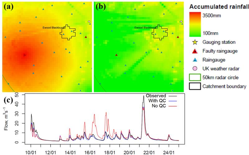
**Fig. 3** Accumulated rainfall in the vicinity of Blackburn, over 15 days from 10 to 25 January 2008, using raingauge-adjusted radar: (a) without quality-control and (b) with quality-control of raingauge data. (c) Comparison of Grid-to-Grid modelled flow for the River Darwen at Ewood Blackburn using (a) as input (red line) and (b) as input (blue line).
