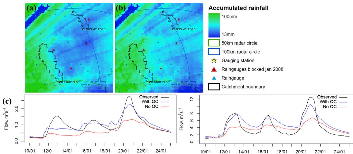
**Fig. 4** Accumulated rainfall in the vicinity of Sudbury, over 15 days from 10 to 25 January 2008, using raingauge-adjusted radar: (a) without quality-control and (b) with quality-control of raingauge data. (c) Comparison of Grid-to-Grid modelled flow Chad Brook at Long Melford (left) and for the Chelmer at Springfield (right) using (a) as input (red line) and (b) as input (blue line).
