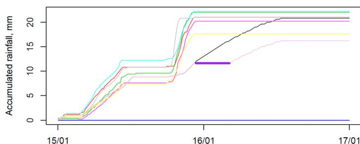
**Fig. 1** Rainfall accumulations showing the effect of a partial blockage on the raingauge at Duston Mill (black line), from 15 to 16 January 2008. Also shown are its nearest seven neighbours (coloured lines), the quality-controlled accumulation (pink line) and the interval identified as suspicious by the tests (purple line). Note that records for the gauge at Litchborough (blue line) were missing for this period.
