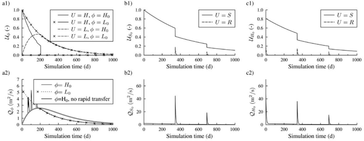
**Fig. 3** Computational example. Graphs (a): hysteresis-based model. Sensitivity of the simulated water levels (graph 1) and of the simulated discharge (graph 2) to  $H_0$  and  $L_0$ . Graphs (b): Fleury model. Sensitivity of the simulated water levels (graph 1) and of the simulated discharge (graph 2) to  $S_0$ . Graphs (c): Fleury model. Sensitivity of the simulated water levels (graph 1) and of the simulated discharge (graph 2) to  $H_0$ .
