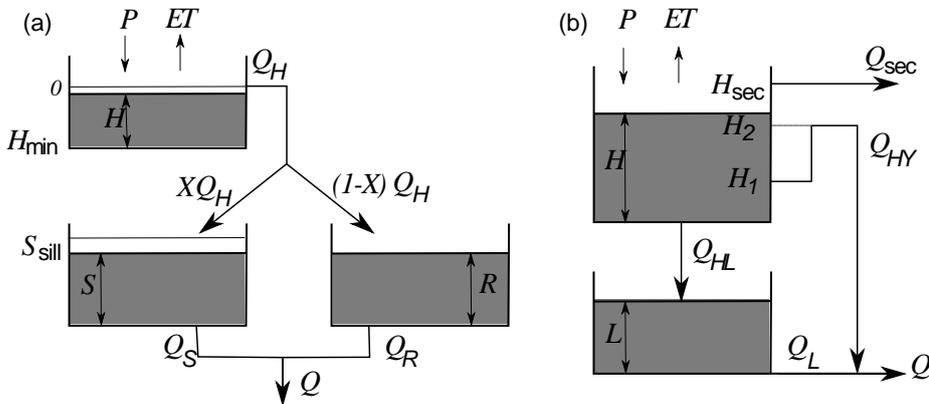
Fig. 1 Structure and notations for: (a) the hysteresis-based model, (b) the Fleury model.
