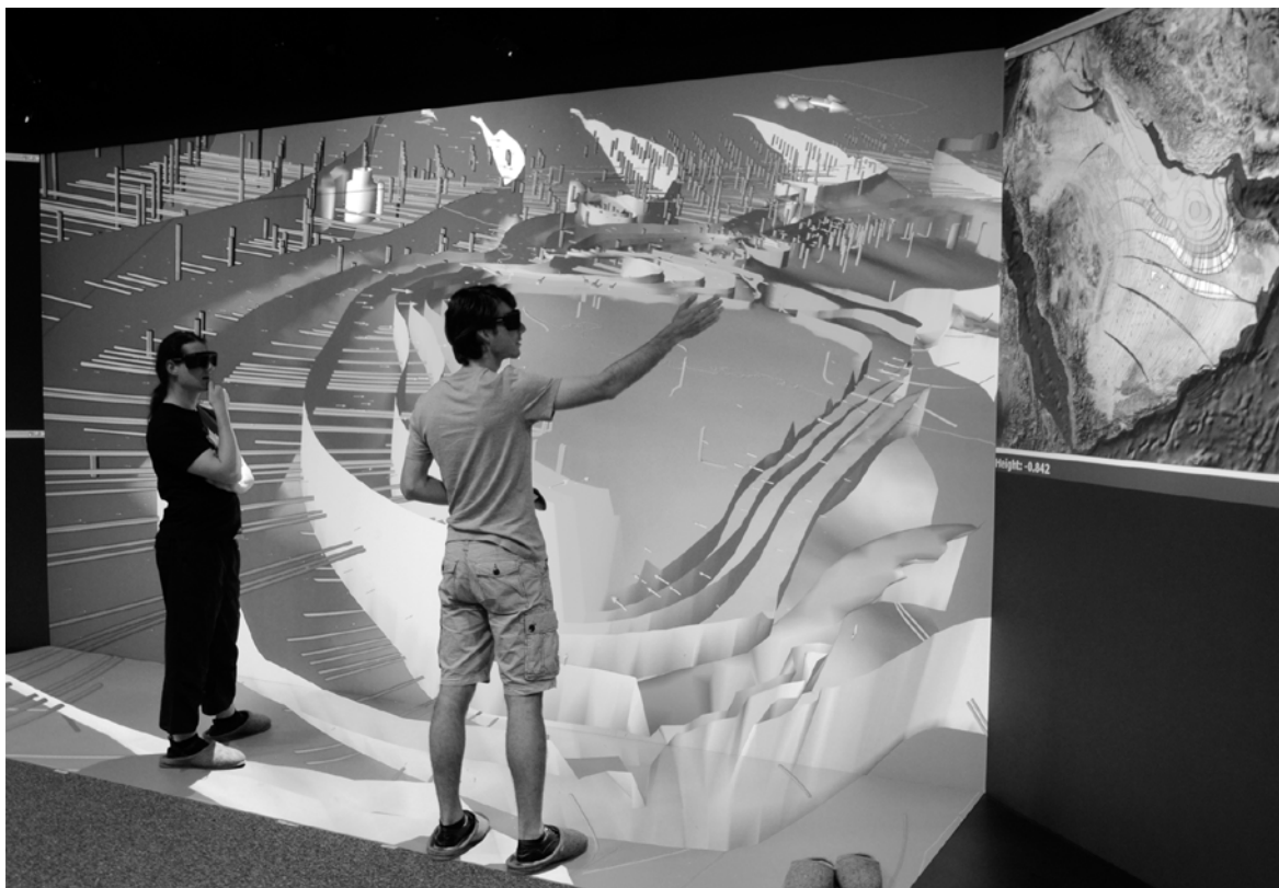
Fig. 4 Two people discussing the simulation results that are shown as 3D stereoscopic visualization on the rear screen and on the floor using isosurfaces to show the hydraulic head and streamlines to indicate the flow direction. Vertical line structures indicate the boreholes and wells. On the right a 2D view that shows a map of the Arabian Peninsula.
