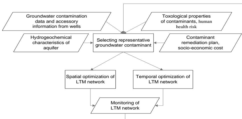
**Fig. 1** Conceptual flowchart of groundwater monitoring network optimization.
