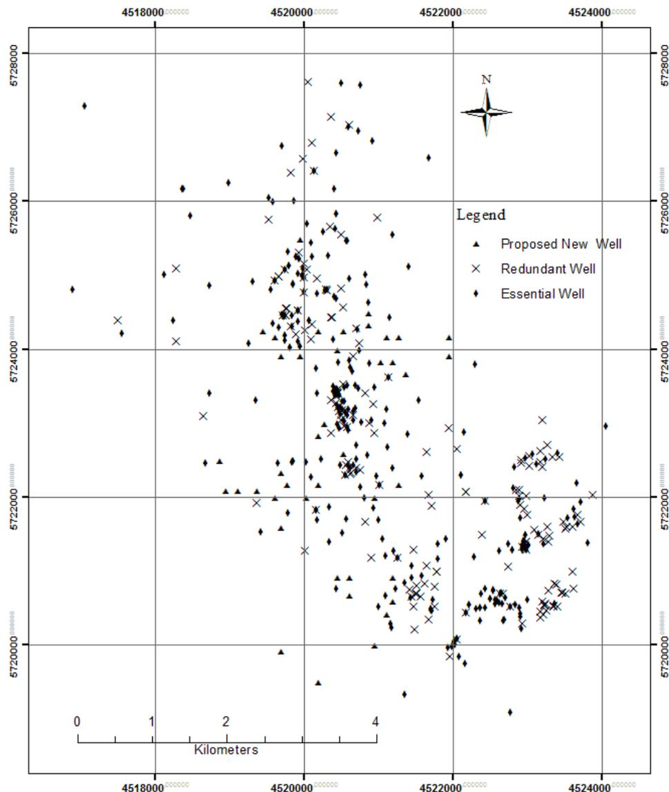
**Fig. 3** Optimized LTM network map showing essential, redundant, and proposed new wells.
