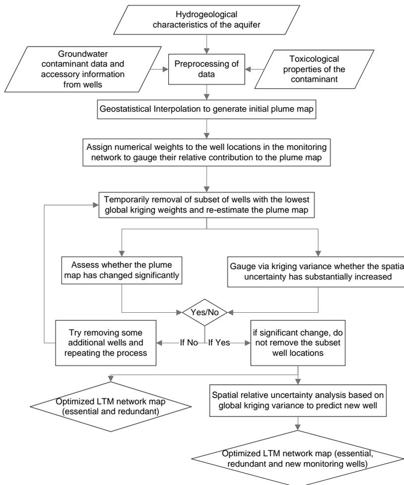
**Fig. 2** Research steps to locate essential and redundant wells and to propose new wells in the existing monitoring network.
