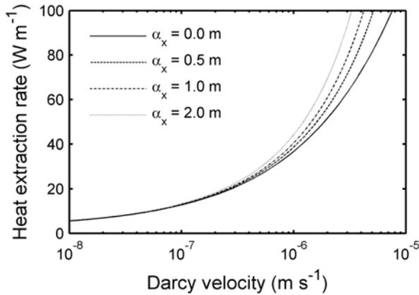
**Fig. 2** Energy extraction needed to result in a temperature change of 1.0 K at 10 m downgradient from the source. The y-axis provides possible energy extraction values for one borehole heat exchanger.
