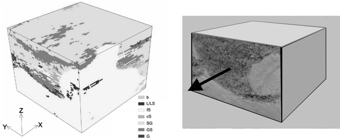
**Fig. 1** Left: example of the facies distribution for a sedimentary block of about  $3 \text{ m}^3$ , as obtained after steps (a) to (d). Right: sketch of the geometry and the boundary conditions to simulate conservative convective transport along the  $x$  direction (shown by the arrow); no flow boundary conditions are assigned on the lateral sides.
