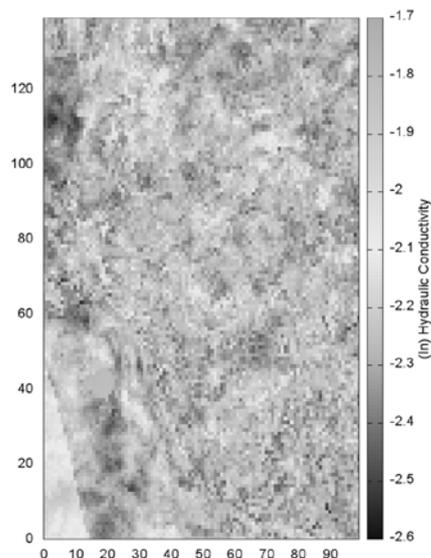
**Fig. 1** Plan view of ensemble averaged stochastic field of (ln) hydraulic conductivity at the surface.
