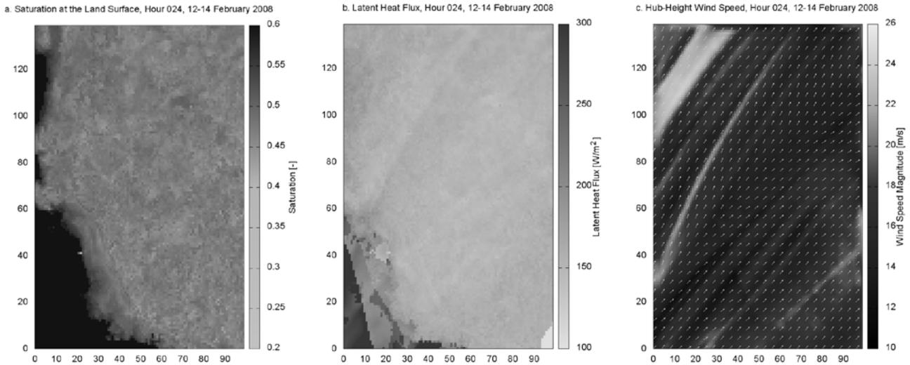
**Fig. 2** Ensemble average timeslices at peak wind speed for the FEB08 ramping event: (a) saturation at the land surface; (b) latent heat flux; (c) hub-height wind speed.
