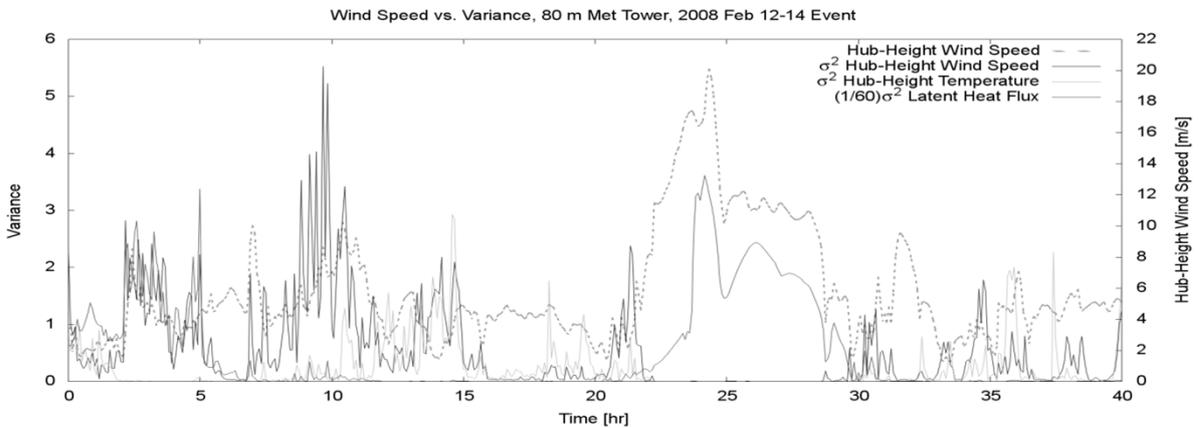
**Fig. 4** Comparison of variances of latent heat flux, hub-height air temperature and hub-height wind speed for the FEB08 ramping event at: (a) the 80-m meteorological observation tower, (b) the 50-m observation tower and (c) the sodar.
