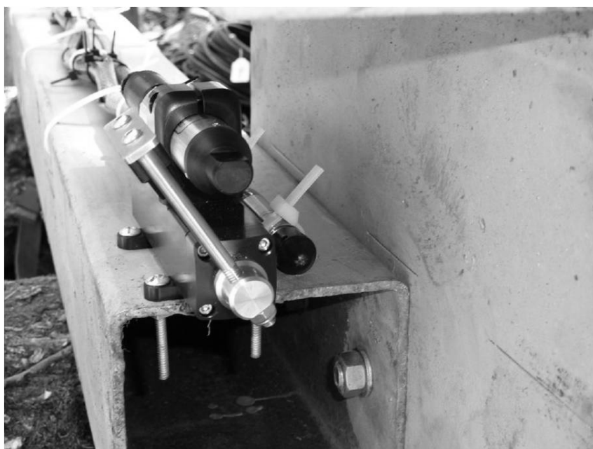
Fig. 2 The steel manifold at the Sepu monitoring station (5°27.8'S, 145°12.6'E) supporting and protecting an OBS-3+SB-2.5-T4 turbidity probe and self-cleaning Hydro-Wiper device (centre left) plus a Druck PDCR1830 pressure transmitter (centre) for monitoring river stage. The unit is shown prior to its insertion into the river.
