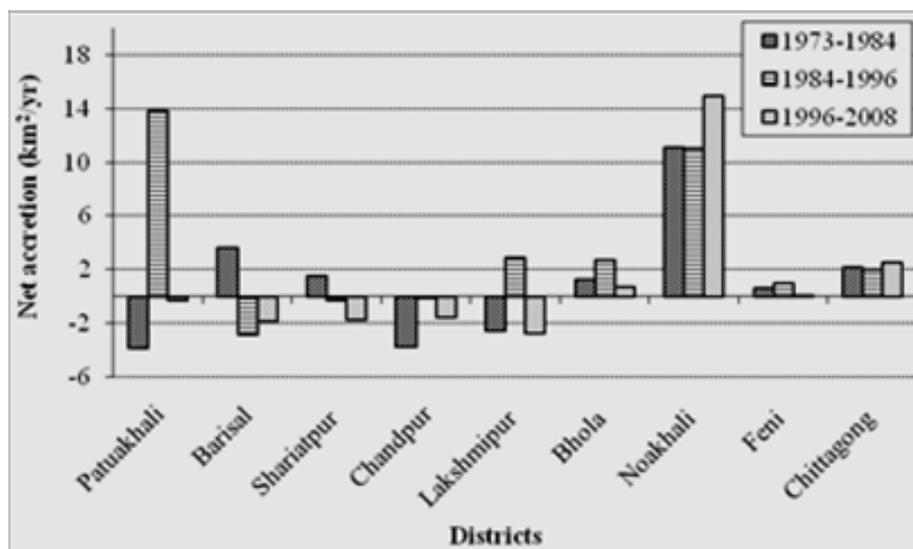
Fig. 7 The spatial distribution of erosion and accretion in the erosion/accretion process.
