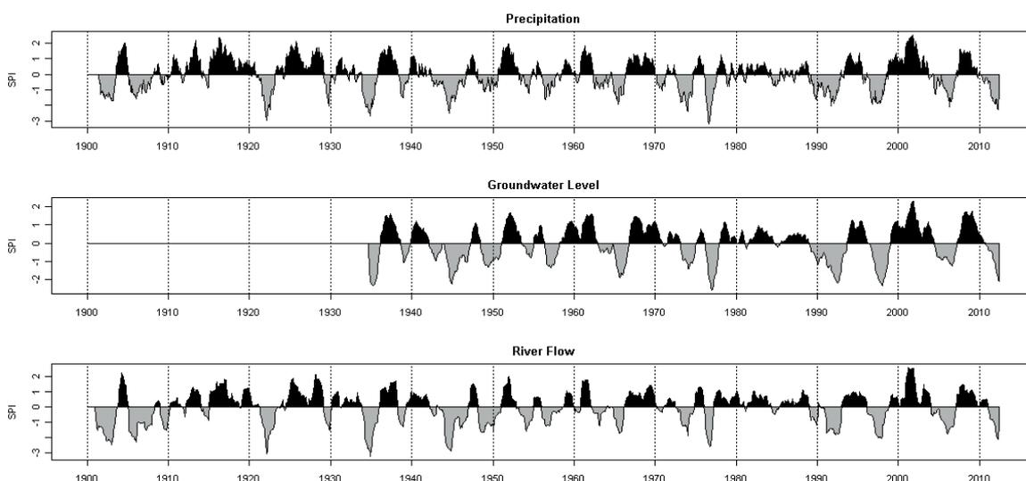
**Fig 3** SPI-based droughts for the Thames catchment, using SPI18 for precipitation, and SPI12 for groundwater levels (Rockley borehole) and river flow (Thames at Kingston, UK).
