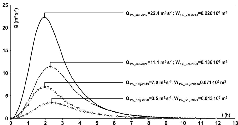
**Fig. 4** Computed hydrographs of maximal discharges into the Kaljavi and Jezeovac streams (under conditions before and after restoration of the “blue-green” corridors).
