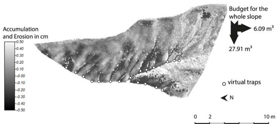
Fig. 2 Erosion and accumulation estimates for the hill slope in the Lainbach valley from July 2009 to Oct. 2013. The arrows indicate the amount of material deposited on the slope and transported out of the study area. “Virtual traps” at the bottom of the gullies are represented by circles.
