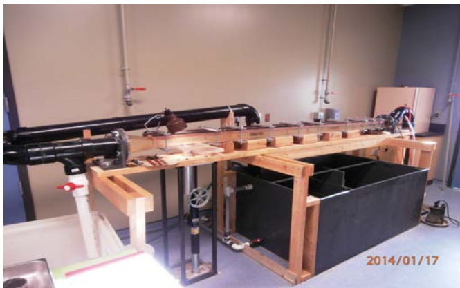
Fig. 4 Erosion measurement device.
