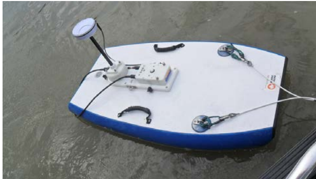
Fig. 3 M9 ADCP River Surveyor from the University of Manitoba (Kimiaghalam et al. , 2013).
