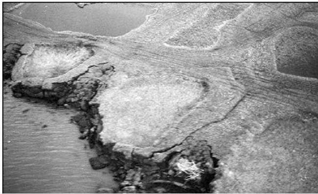
Fig. 3 High level ice wedge polygon pond drained because of riverbank erosion.
