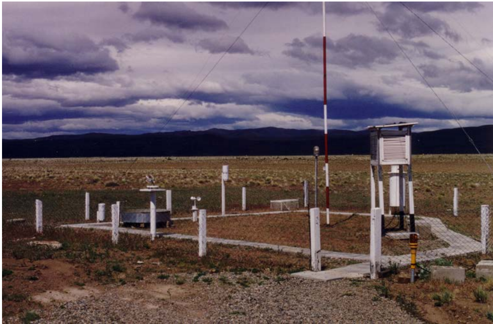
Plate 4.1 Meteorological station at Esquel, Patagonia. From left to right: raingauge, evaporation pan, solarimeter, anemometer, raingauge, radiometer, anemometer mast, and Stevenson screen with recording raingauge behind.
