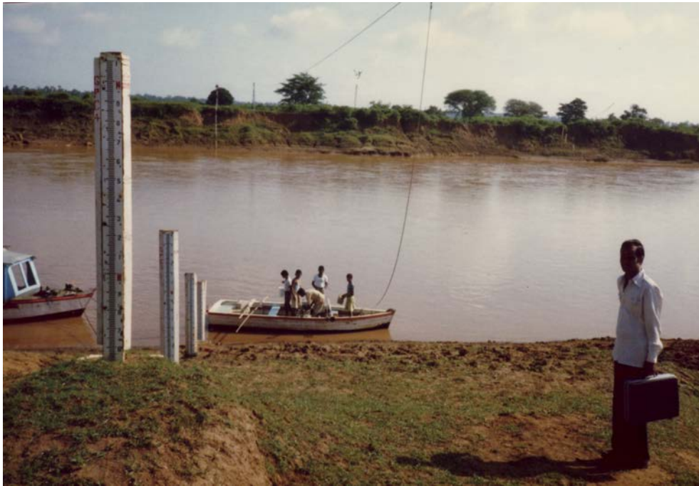
Plate 7.1 Gauging station, including staff gauges and a cableway, on the River Indravati at Jagdarpur, central India.
