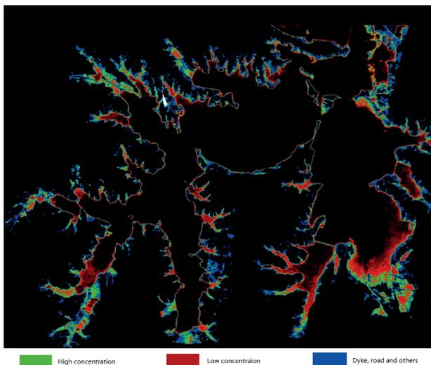
**Fig. 5** Cyanobacteria bloom NDVI after FLAASH atmospheric correction.
