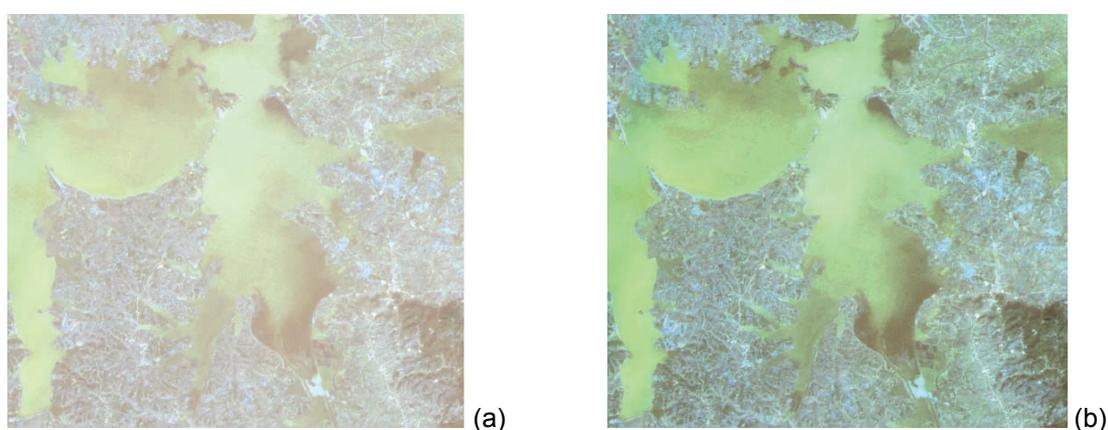
**Fig. 2** Result of comparison of before and after FLAASH atmospheric correction; (a) before atmospheric correction, and (b) after atmospheric correction.
