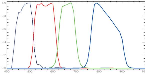
Fig. 1 Spectral response function of HJ-1A CCD2.
