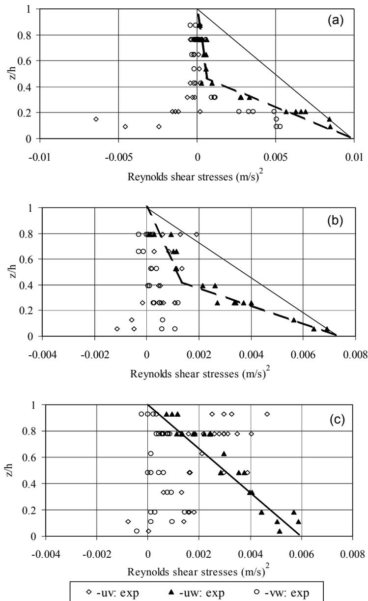
**Fig. 5** Reynolds shear stress from ADV data. (a)  $y = 23.95$  (m); (b)  $y = 25.0$  (m); and (c)  $y = 27.0$  (m). The dashed lines indicate the vertically double-layer flow structure, and the solid lines correspond to linear distributions valid for single channel flows.
