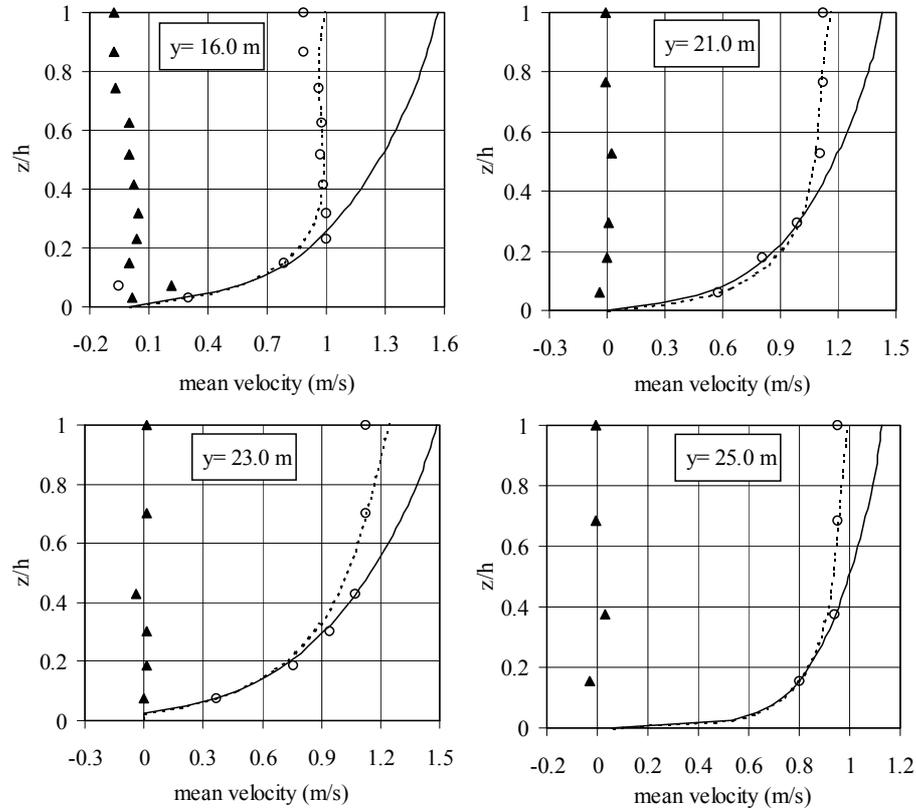
**Fig. 3** DCM (symbols) and computed (lines) mean velocities on selected verticals. The solid lines correspond to  $\Pi \equiv 0.2$ , and for dashed lines  $\Pi$  is given in Table 1.
