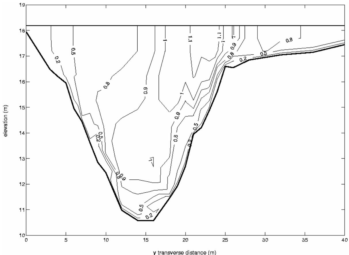
Fig. 4 Isovells of DCM streamwise velocity ( $\text{m s}^{-1}$ ).
