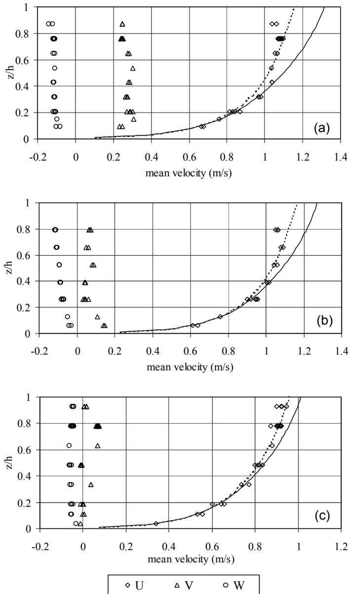
**Fig. 2** ADV (symbols) and computed (lines) mean velocities. (a)  $y = 23.95$  (m); (b)  $y = 25.0$  (m); and (c)  $y = 27.0$  (m). The solid lines correspond to  $\Pi \equiv 0.2$ , and for dashed lines  $\Pi$  is given in Table 1.
