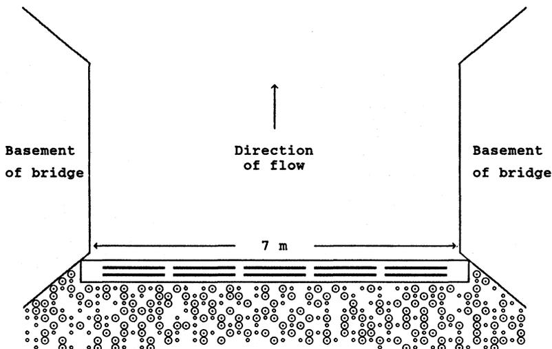
Fig. 2 View of the detector log at Squaw Creek, Montana, USA.
