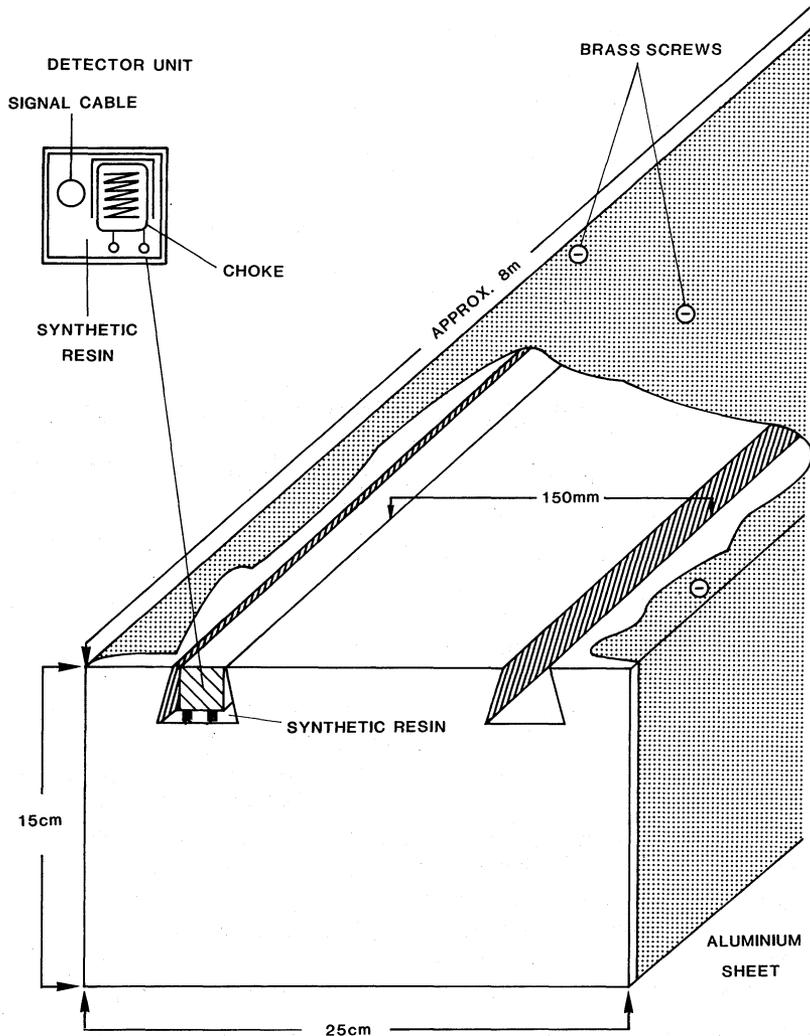
*Fig. 1* Cross section of the detector log.
