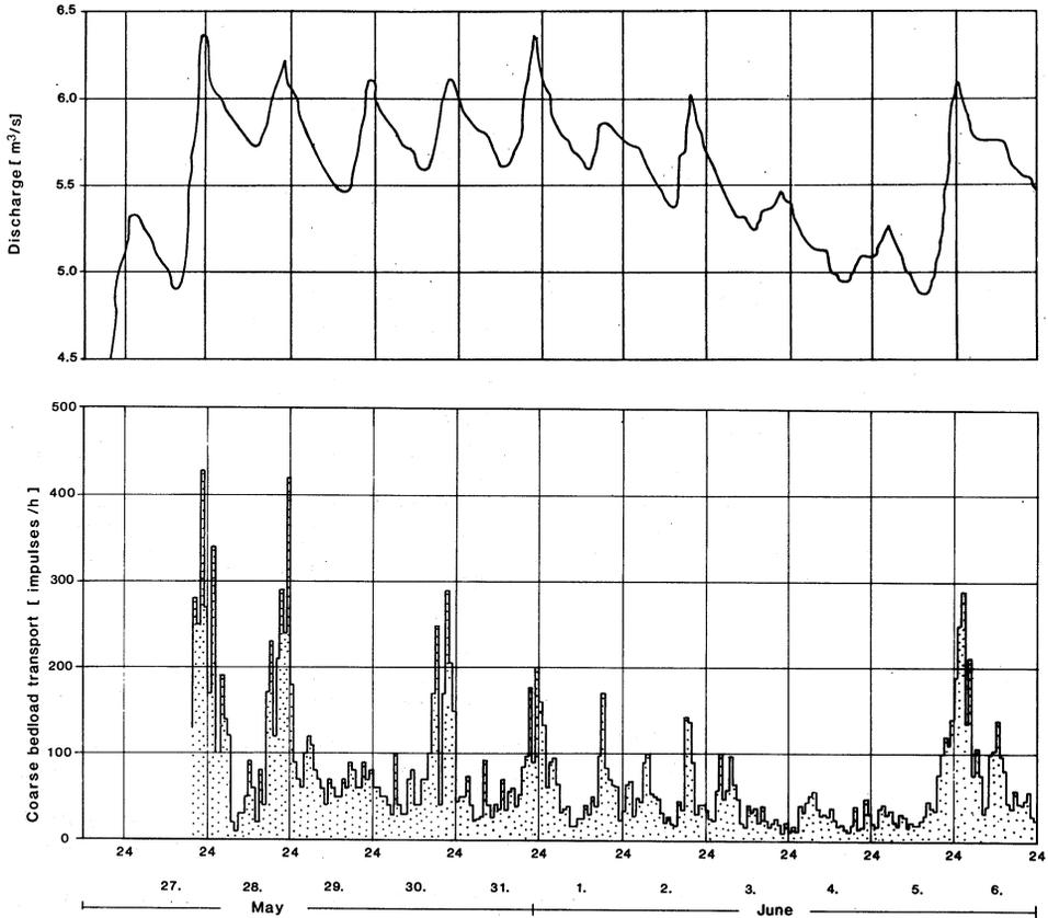
*Fig. 5 Discharge hydrograph versus coarse material transport (in counts per hour) (from Bunte et al., 1987).*
