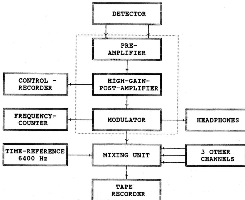
Fig. 3 Block diagram of recording electronics.
