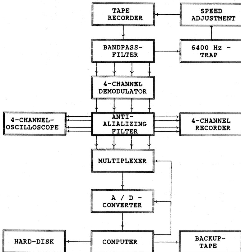
Fig. 4 Block diagram of demodulation and A/D-conversion.
