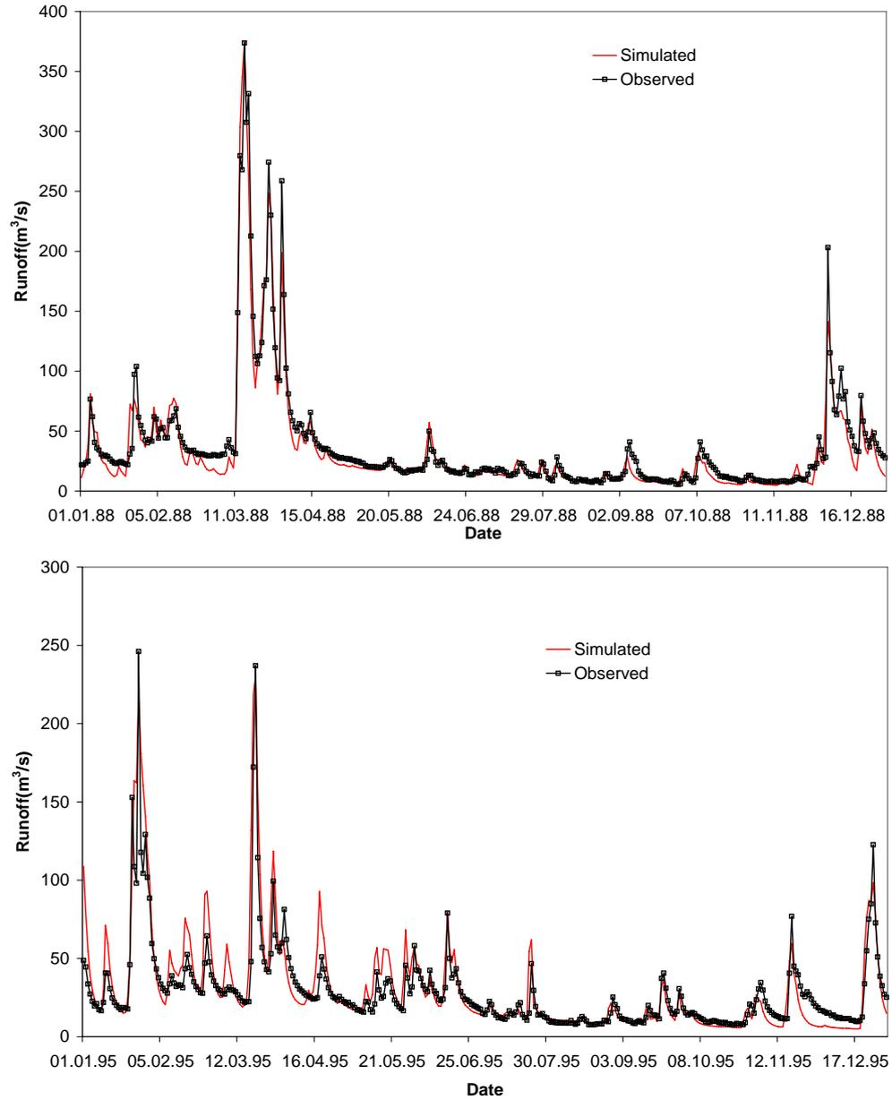
**Fig. 2** Simulated and measured runoff at the outlet of the Kocher catchment shown for 1 year in the calibration period (upper graph) and validation period (lower graph).
