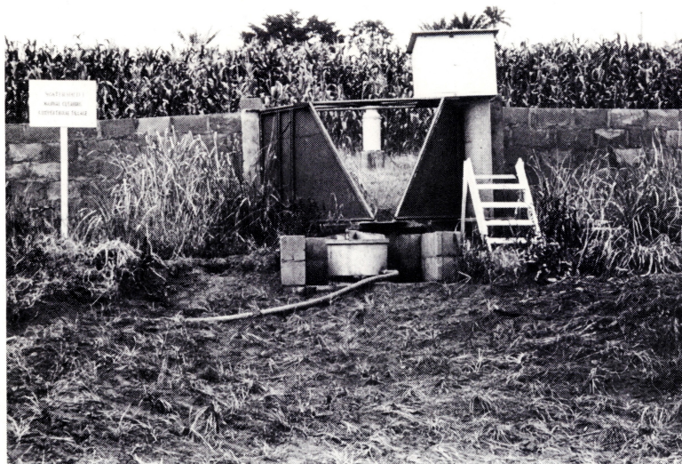
FIG.4 H-Flume with a water level recorder (white box) and a Coshockton sampler.
