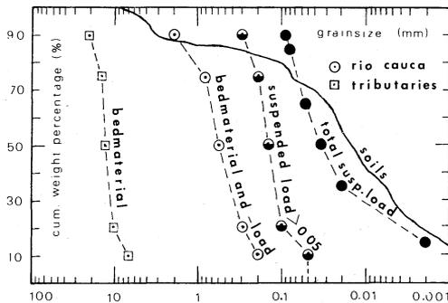
FIG.2 Typical grain size distributions in the Cauca basin. Note that all curves are approximate, except for soils.
