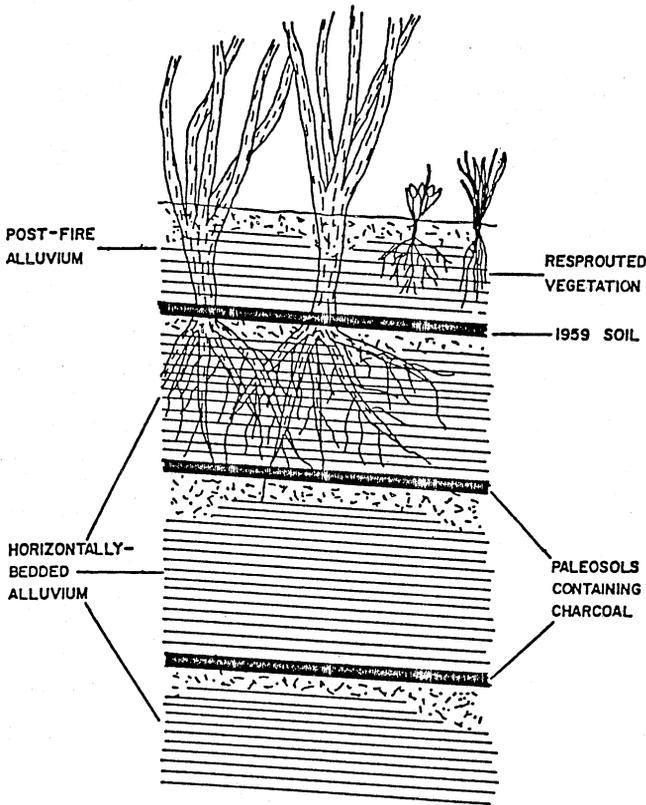
Fig. 4 Idealized diagram of horizontally-bedded alluvium and intervening paleosols in El Oso Creek alluvium.
