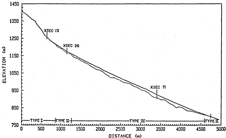
Fig. 5 El Oso Creek longitudinal profile and sub-alluvial bedrock profile. The channel is divided into the three reach types. A representative cross-section of each is shown in Fig. 6.
