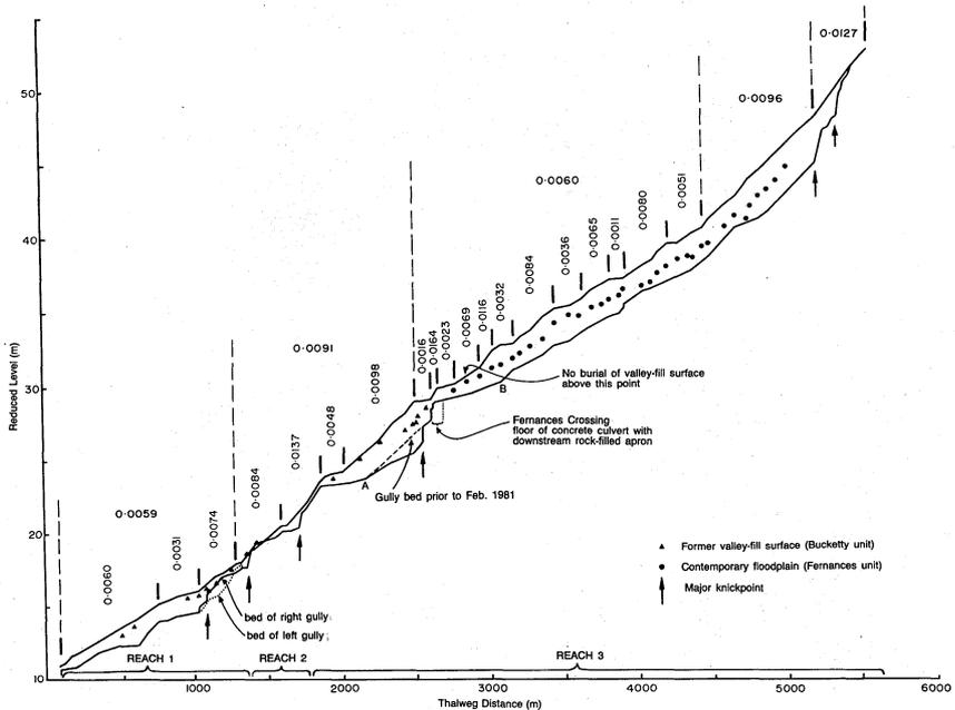
FIG. 3 Field-surveyed longitudinal profile of lower Fernances and Finchs Creeks. Slopes (m/m) shown as numbers above present valley floor.
