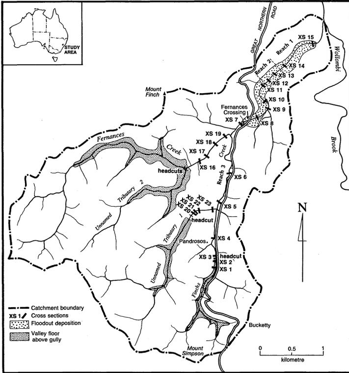
FIG. 1 Location of Fernances Creek drainage basin showing the valley network, gully reaches and surveyed cross sections.
