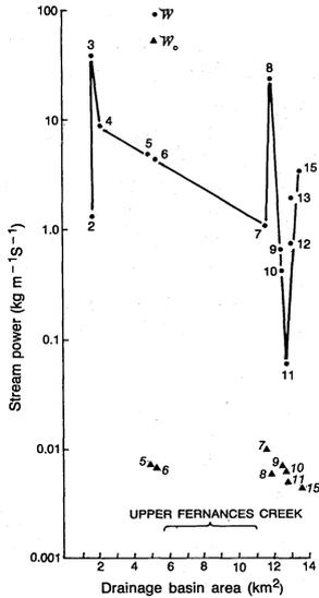
FIG. 4 Computed values of unit stream power ( $\omega$ ) and threshold unit stream power ( $\omega_0$ ) for sediment transport as a function of basin area in Finchs and Fernances Creek at each of the numbered cross sections.
