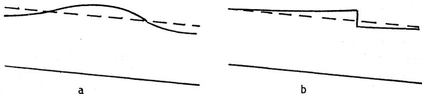
FIG. 2 Undular (a) and breaking (b) surges
