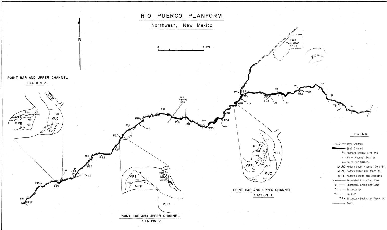
FIG. 2. Planform map of the Rio Puerco study area showing: (1) the 1945 and 1978 channel of the Rio Puerco, (2) cross-section locations, and (3) sediment-sample station locations. Note stream flow is from east to west.
