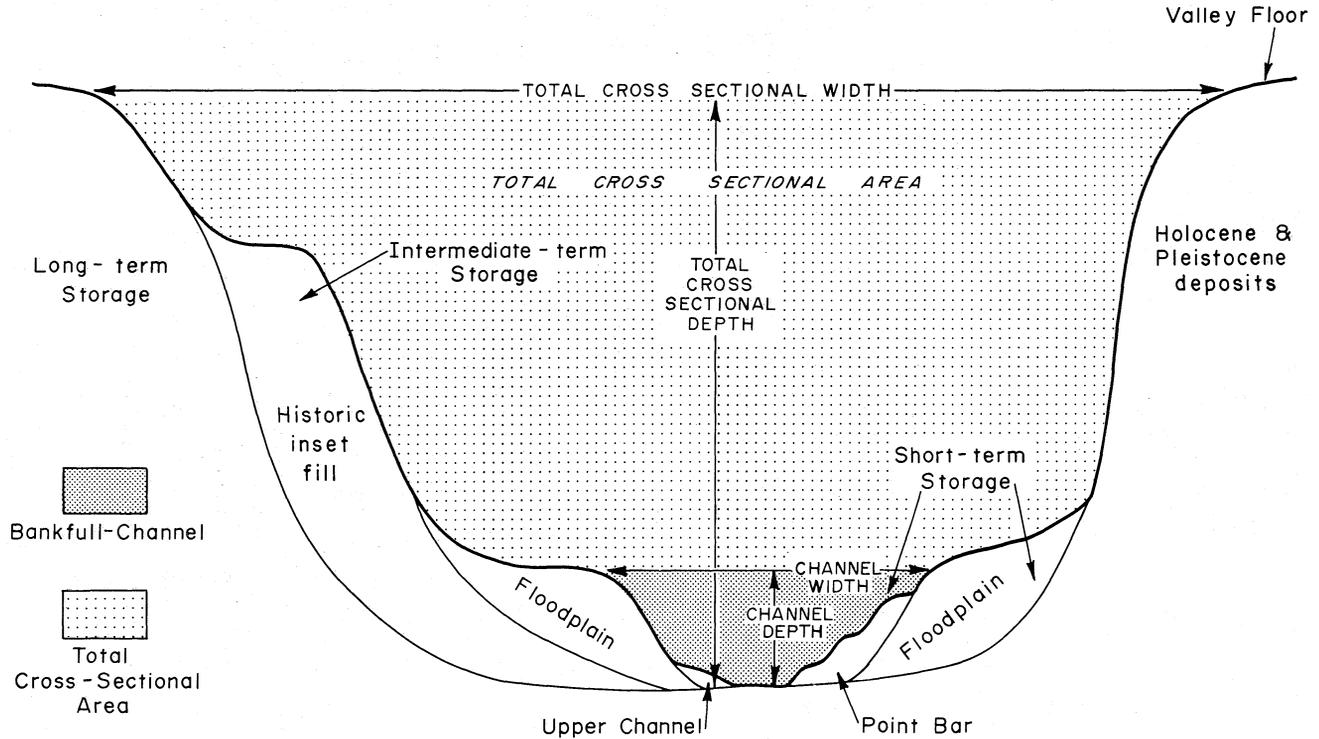
FIG. 3. Diagrammatic cross section showing: (1) channel morphology measurements, (2) differences between total and bankfull cross-sectional area and (3) long-term, intermediate-term, and short-term storage sites along the Rio Puerco.
