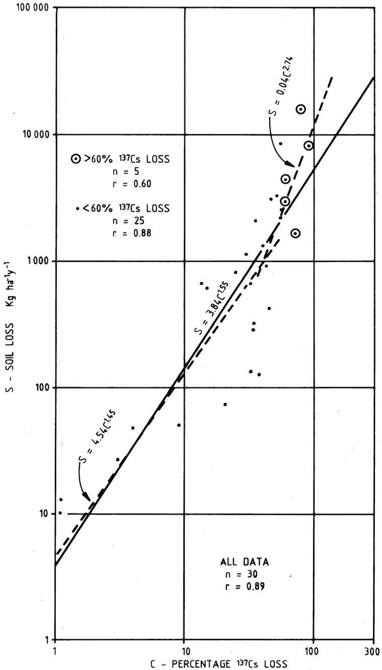
FIG. 3 Soil loss v. caesium-137 loss for runoff - erosion plots in eastern New South Wales
