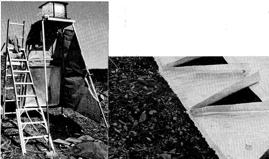
**Fig. 2** Rainfall simulator and overland flow collection system.
