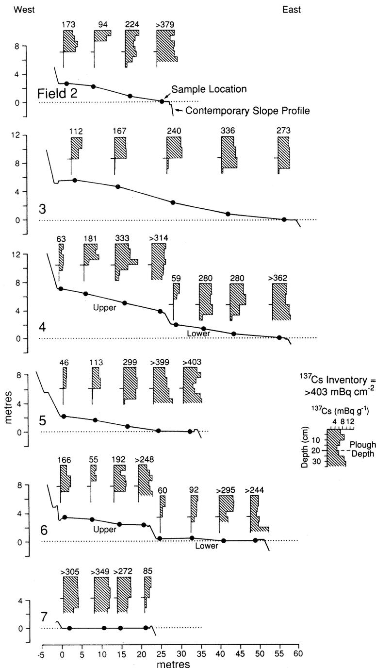
Fig. 3 Slope profiles, sampling locations, caesium-137 inventories and depth distributions for the sampled fields, near Yanting.
