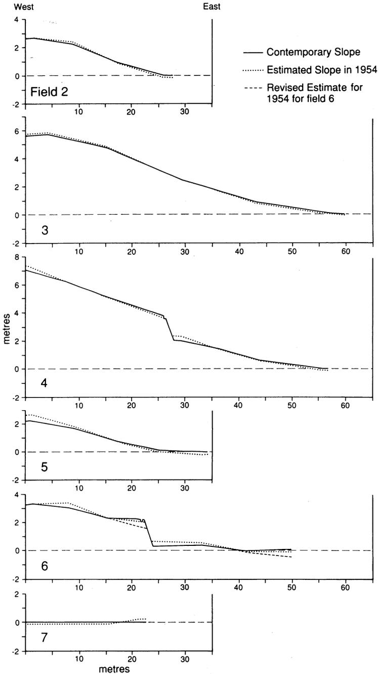
**Fig. 4** The pattern of erosion and aggradation illustrated by comparison of the contemporary slope profiles with their estimated form in 1954. The two estimates for field 6 are discussed in the text.
