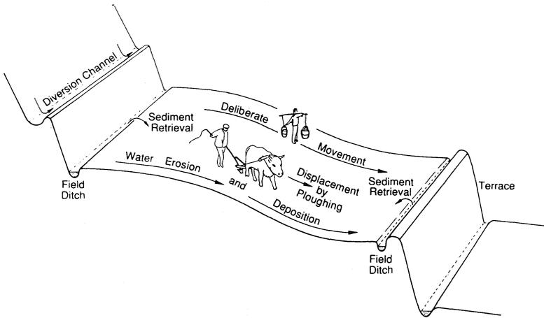
Fig. 2 Schematic diagram of soil conservation measures and processes of soil redistribution in a terraced landscape at Yanting.
