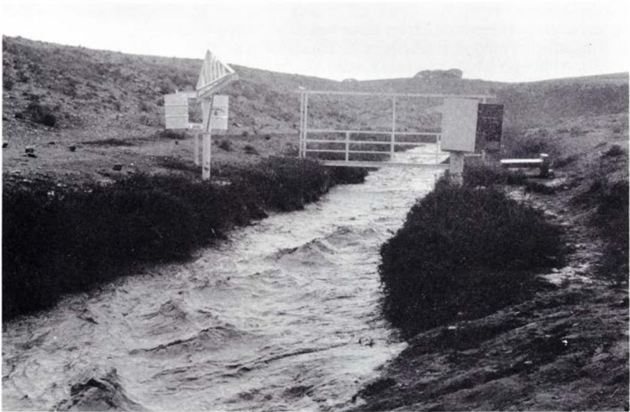
FIG. 2 View of the Nahal Yatir during the flash flood on 8 February 1991, showing swivelling davit, sampling bridge and instrument housing at the sediment transport monitoring station.
