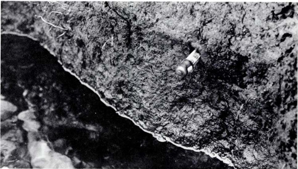
FIG. 4 A PEEP sensor emerging from the bank face at the Upper Severn site. The reference cell and two cells in series can be seen (photo: A. James).
