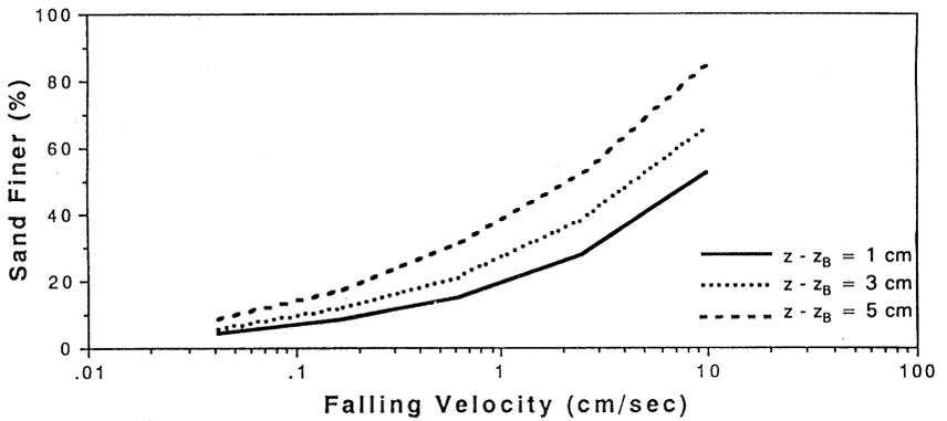
Fig. 4 Accumulation curves of suspended sediment (RUN-2, 1.5 hour, 6.5 m upstream from weir).
