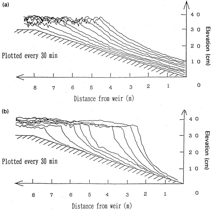
Fig. 2 Bed-profiles of deposited sediment: (a) (RUN-1), (b) (RUN-2).
