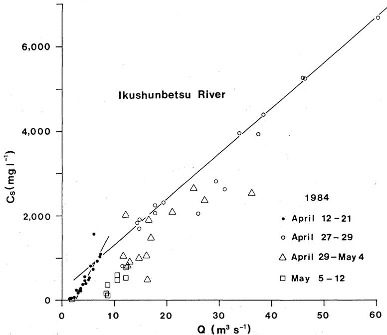
Fig. 6 Total relation between water discharge,  $Q$  and sediment concentration,  $C_s$  for Ikushunbetsu River. The regression line for black circles is the same as in Fig. 5. The line passing through some white circles indicates the possible upper limit of  $C_s$  for give  $Q$ .
