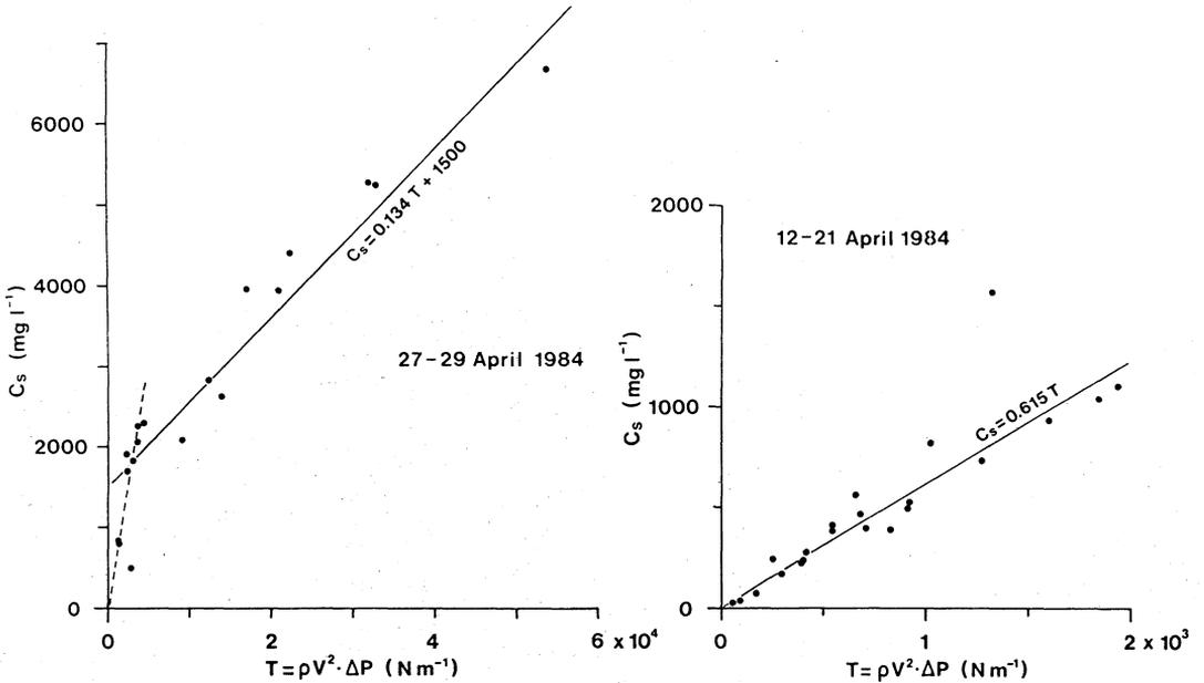
Fig. 7 Relations between the total shear force,  $T$  and sediment concentration,  $C_s$  at the middle snowmelt stage (left) and the first stage (right) of Ikushunbetsu River. The regression line at the first stage is the same as a dotted one at the middle.
