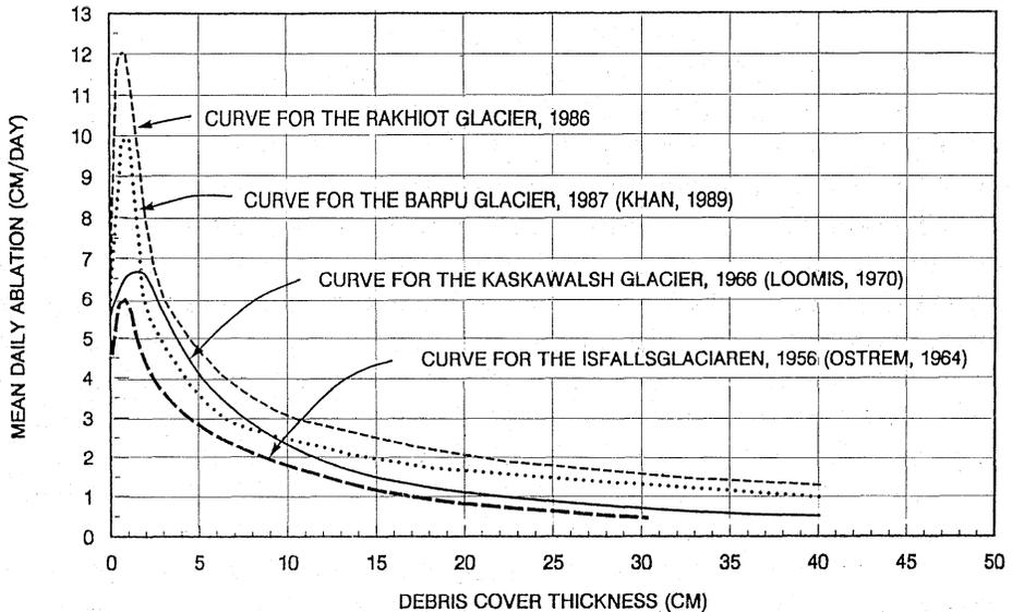
Fig. 1 Relationship between debris cover thickness and ablation.
