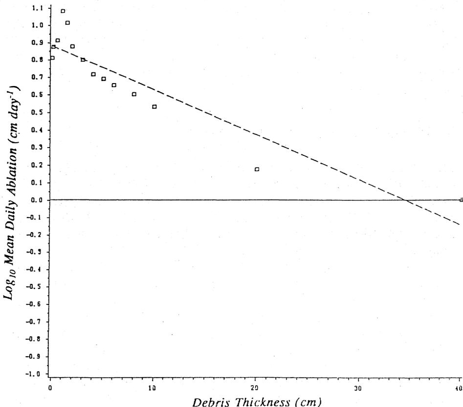
Fig. 2 Scatter diagram relating  $\log_{10}$  mean daily ablation and debris cover thickness.
