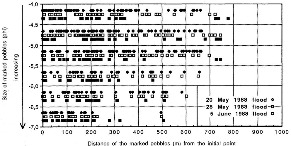
Fig. 4 Distribution of marked pebbles after the floods as a function of their relative size.
