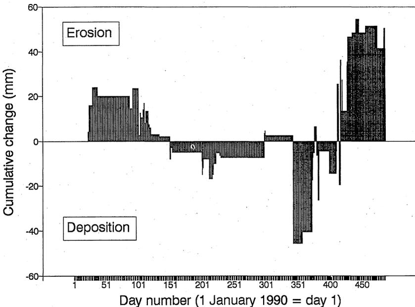
Fig. 6 The pattern of cumulative change at the River Arrow PEEP site 2. A clear seasonal cycle emerges, although erosion and deposition events can occur at any time of the year.
