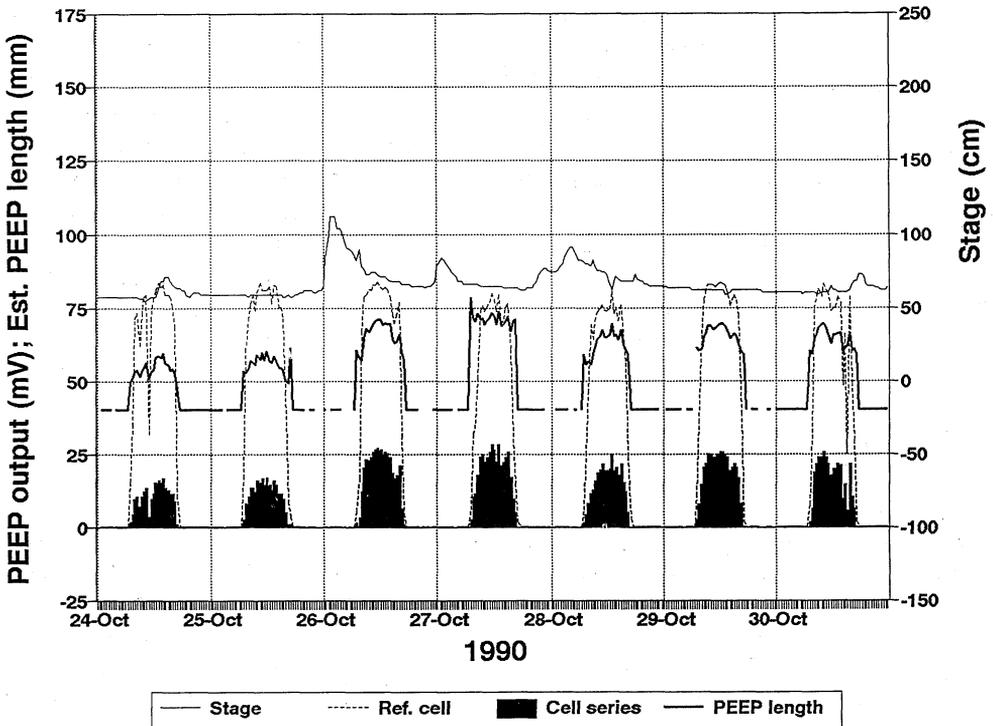
Fig. 1 A moderate flow event on 26 October 1990 producing 11 mm of bank retreat, as detected by the sudden increase in the diurnal trends in PEEP 2 cell series outputs and derived estimated PEEP lengths.
