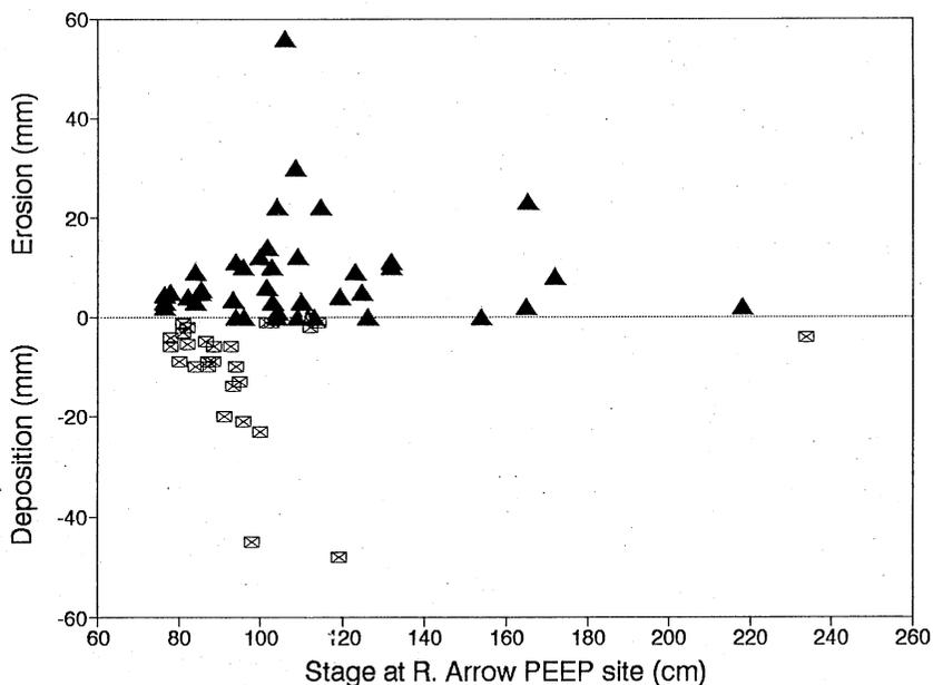
Fig. 3 Relation of peak stage of specific flow rises to the magnitude of associated erosion and deposition events ( $n = 70$ ) on the River Arrow, as recorded by PEEP 2 between January 1990 and May 1991.
