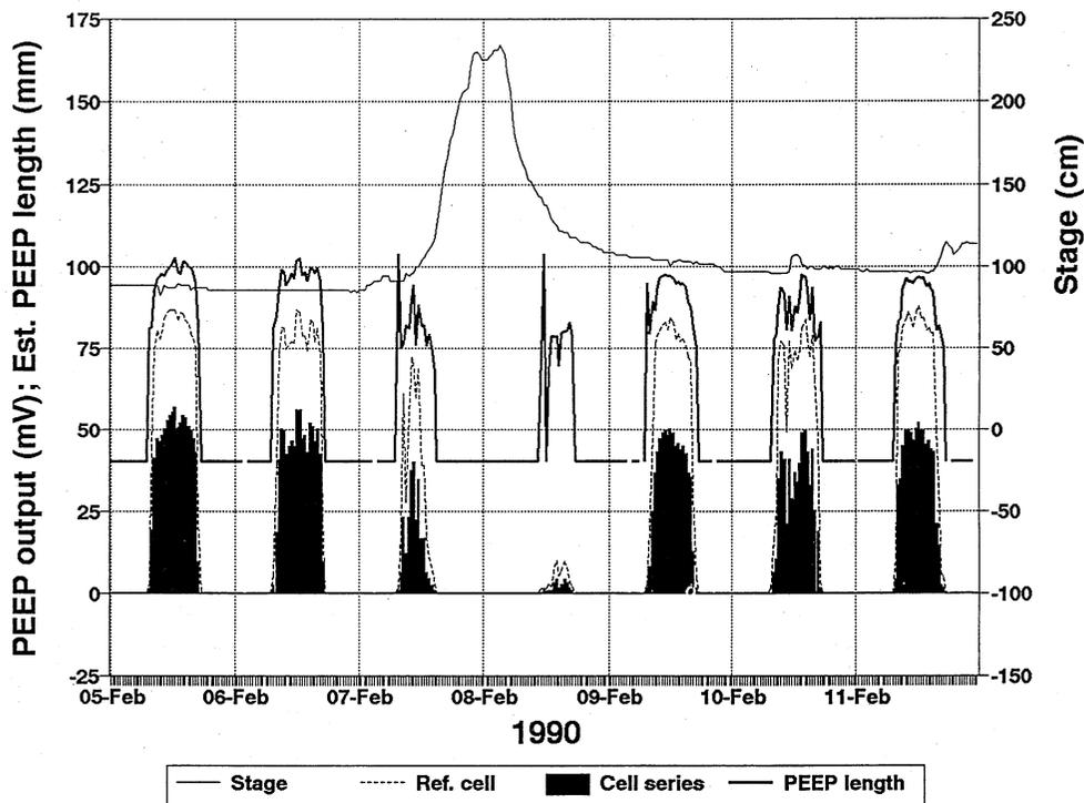
Fig. 2 A very large flow event on 8 February 1990 producing 4 mm of deposition, as detected by the small declines in the diurnal trends in PEEP 2 cell series outputs and derived estimated PEEP lengths (cf. Fig. 1).
