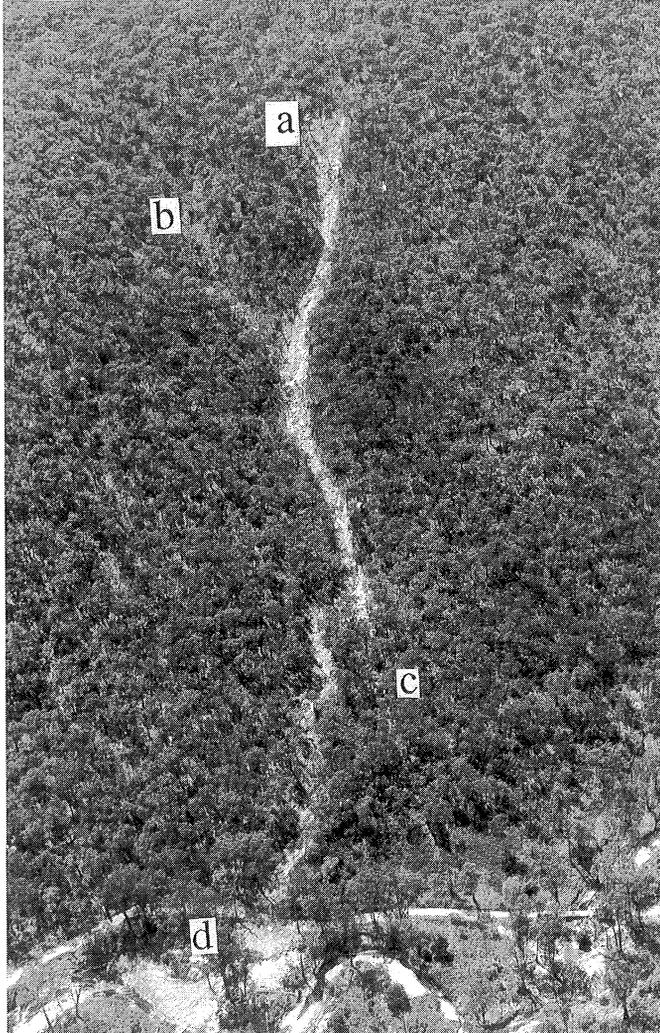
**Fig. 3** Oblique aerial photograph of DF1. Note the following: the rotational slump at the head of the failure (point "a"); the main path of failure does not follow the main drainage line (point "b"); the debris splay visible through the trees below the sharp bend (point "c"); and the fan of material at the junction with Watchbox Creek (point "d").
