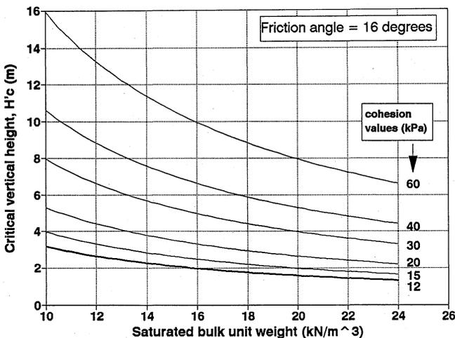
Fig. 2 Culmann-type bank stability curves, predicting critical stable height for vertical banks cut in material of friction angle  $16^\circ$ , for given cohesion values and saturated bulk unit weights.
