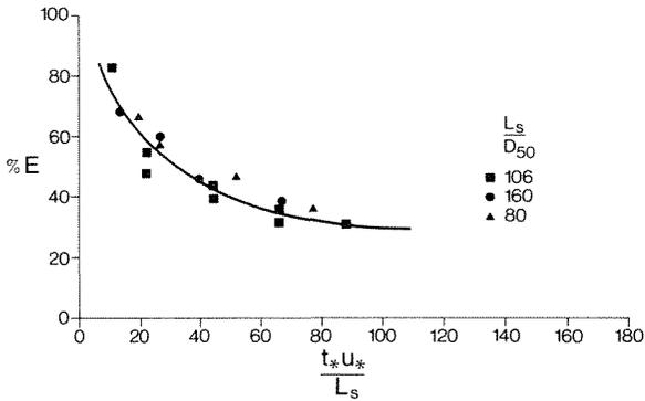
Fig. 3 Efficiency as a function of  $t_*U_*/L_S$  for three values of  $L_S/D_{50}$ .
