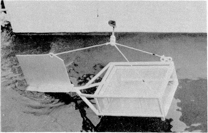
Fig. 1 Basket sampler (courtesy of Water Survey of Canada).
