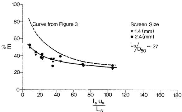
Fig. 4 Efficiency as a function of  $t_*U_*/L_S$  from data by Gibbs (1973).
