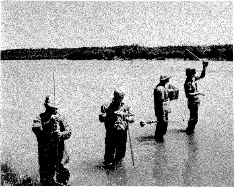
Fig. 1 Field crew taking discharge measurement, collecting suspended samples, and collecting bed material samples on the Niobrara River in Nebraska, USA.
