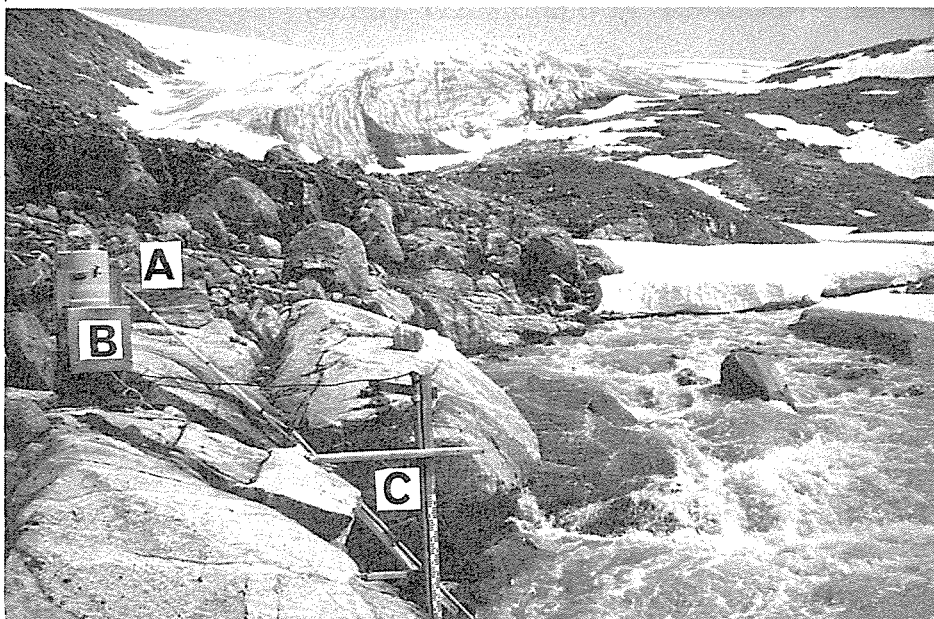
Fig. 3 The sampling station on the Tverrelvskardet stream in Stryn, western Norway. A: ISCO automatic sampler. B: Water level recorder. C: Sampling tube and pressure transducer.
