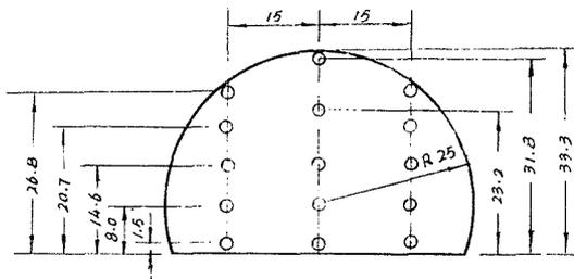
Fig. 3 Sectional drawing of the layout of the points for velocity measurement inside the sampler container (all dimensions are in mm).
