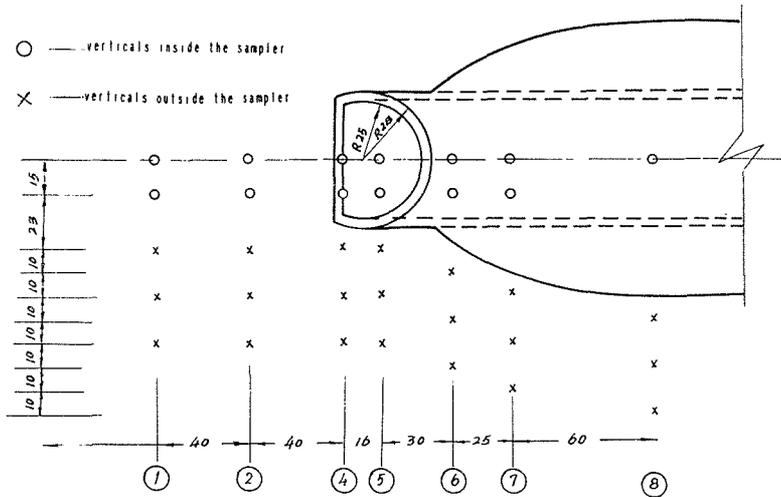
Fig. 2 Plan of the layout of the points for velocity measurements around the sampler (all dimensions are in mm).
