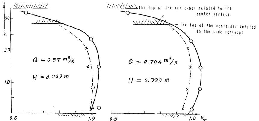
**Fig. 4** Distribution character of velocities of the sampler container.
