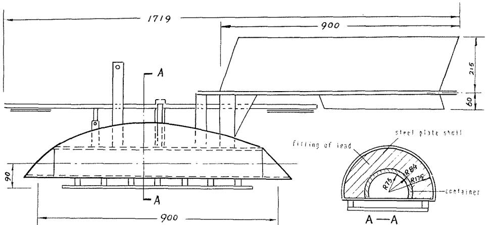
Fig. 1 The NBS-84 near-streambed suspended load sampler.
