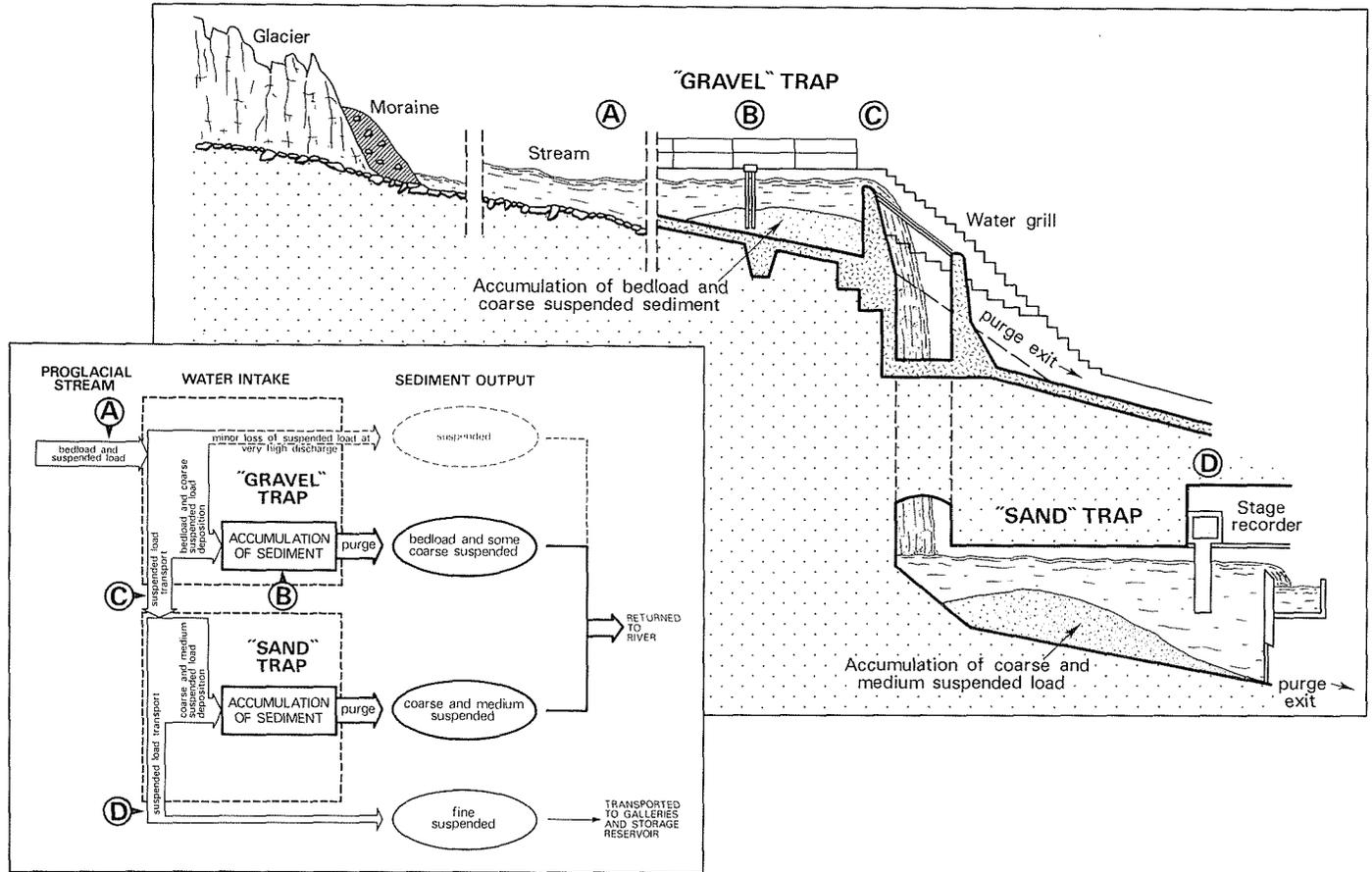
Fig. 1 Sketch and flow diagram of the sediment trapping and purging mechanism of the meltwater intake structures.
