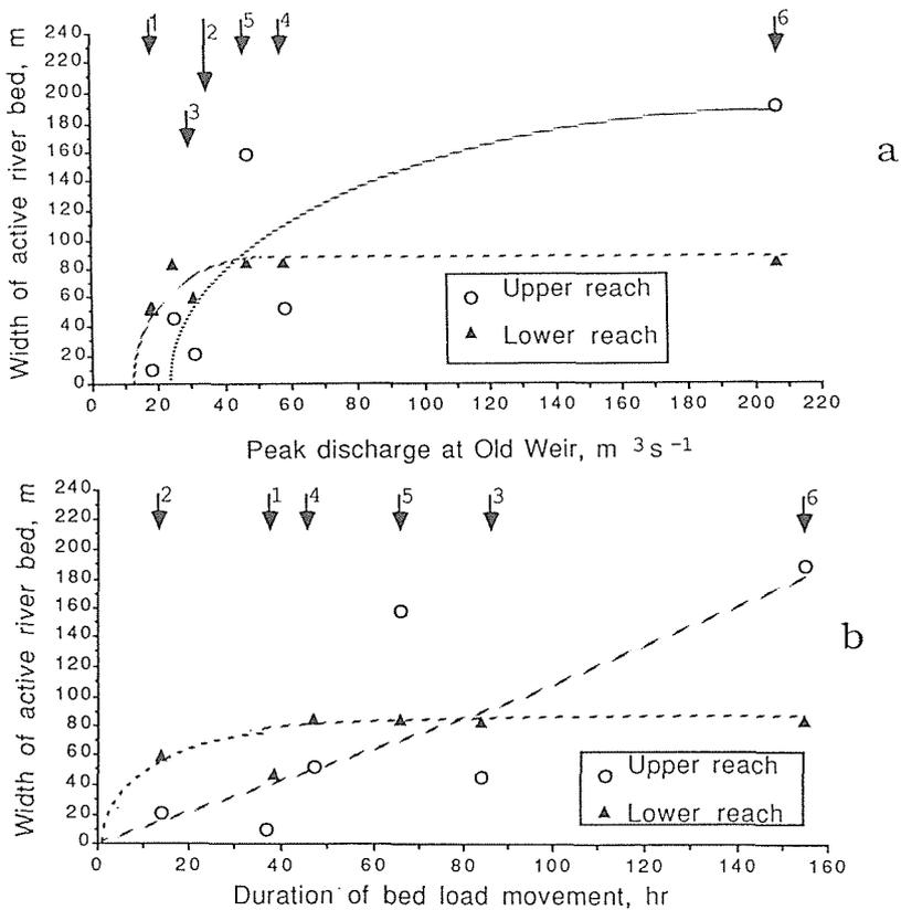
**Fig. 2.** Width of bed activity vs. peak discharge (a) and vs. duration of bedload movement (b). The numbers denote the six successive flow events monitored during December 1985 - March 1986.
