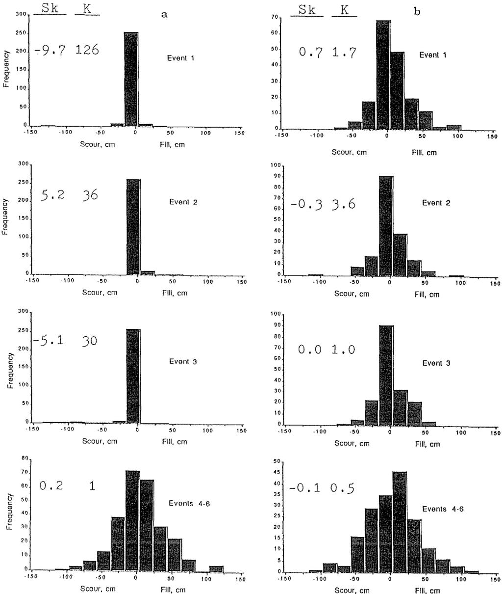
**Fig. 3.** Frequency distributions of net resurvey scour and fill in the upper (a) and lower (b) study reaches, North Branch Ashburton River.
