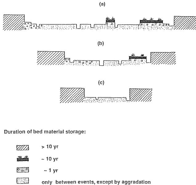
**Fig. 4.** Schematic cross sections depicting storage potential of a braided (a), slightly confined (b) and considerably confined reach (c).
